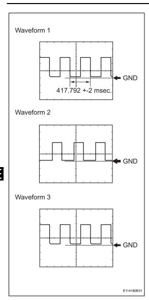
(a) Using an oscilloscope, check the signal waveform of the meter.
