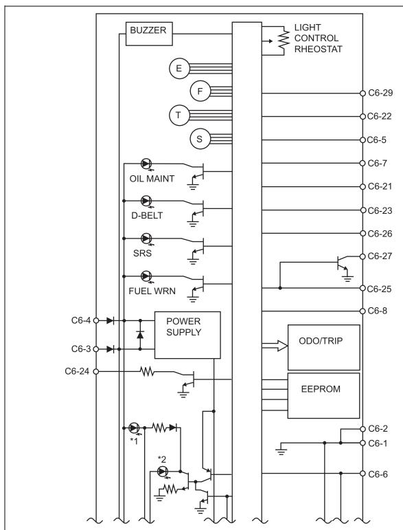
F: Fuel Gauge, T: Tachometer, S: Speedometer, E: Engine Coolant Temperature Gauge \*1: ODO/TRIP Illumination, \*2: Except ODO/TRIP Illumination
