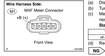
a) Disconnect the M1 Mass Air Flow (MAF) meter connector.
