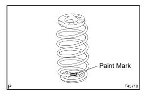
(b) Install the rear coil spring insulator lower and the coil spring rear LH to the rear axle beam.
