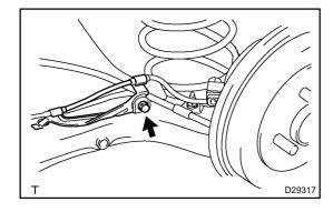
(b) Remove the bolt and separate the skid control sensor wire from the axle beam.
